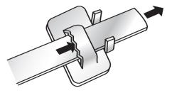
Pull appropriate length of band from BAND-IT Tote (approx. 3 1/2 times the diameter of the pole or mastarm for a single-wrapped clamp and seven times the diameter for a double-wrapped clamp. Add 6-8 inches for both single-wrapped and double-wrapped clamps to accommodate the tail and bracket design.) Cut the band using one of the BAND-IT tools with built-in cutter. One end of the band will be very flat and the opposite end will be slightly bent from the cut-off.
