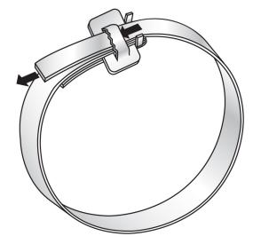
4. Wrap band through sign bracket and around the pole or mastarm and thread through bridge as shown.
