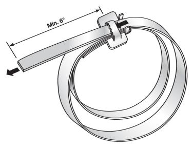
5. Repeat a second wrap of band through the bracket and buckle for a continuous double-wrap application. Double-wrapping develops greater radial compression than single-wrapped clamps and more than doubles the holding strength for heavy objects and high wind loads.
