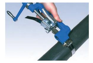
6. Place band in open slot of tool nose and gripper block. Move into slot as far as possible to prevent buckle from sliding into tool nose. With thumb on band gripper lever, apply tension by turning handle of tool. After tension is created, it is no longer necessary to hold the band gripper lever as it locks itself under tension. When band stops moving through buckle, maximum tension has been applied. Stop turning handle.
